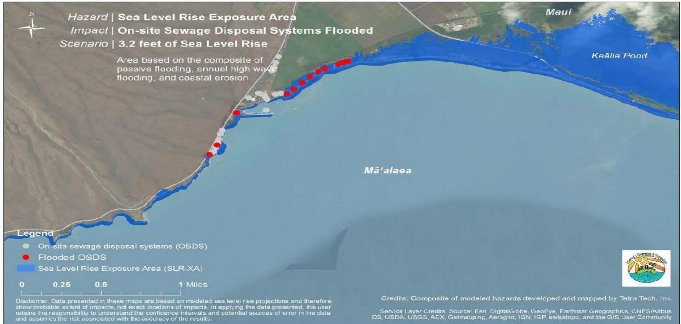
Figure 67. On-site sewage disposal systems flooded in the SLR-XA with 3.2 feet of sea level rise along Mā'alaea, Maui
