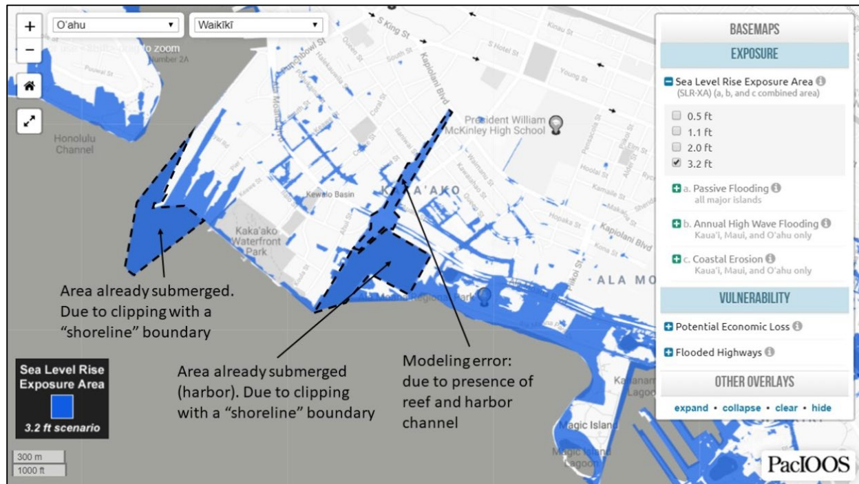
Figure 4. Modeling errors in the annual high wave flooding model (and combined SLR-XA) are found at a limited number of shoreline areas landward of natural and artificial channels in the nearshore reef (example from Ala Moana and Kaka‘ako, O‘ahu). Also shown in this figure are clipping errors, which are mapping artifacts that identify offshore submerged areas as being flooded by sea level rise. These artifacts result from clipping of the SLR-XA map data using a shoreline boundary (Special Management Area), which in some areas differs from the natural shoreline.
