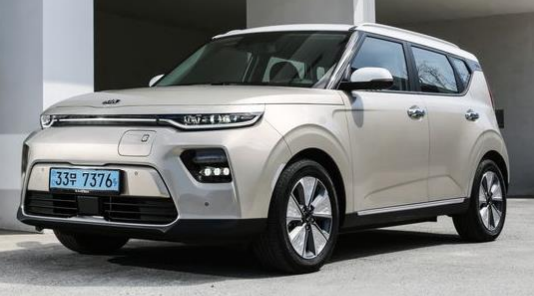
2020 Kia Soul EV 243-mile range 64kWh battery Estimated base $37,500
