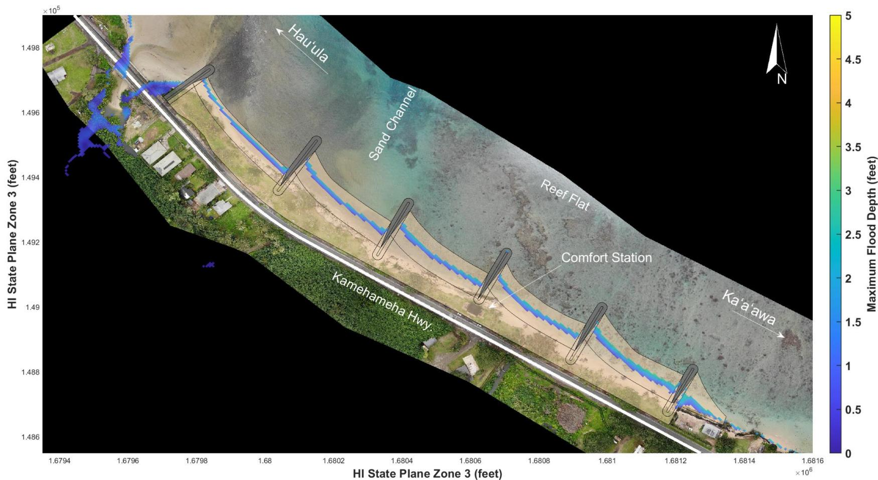
Figure 11-9. Maximum modeled flood depth for the partially stabilized pocket beaches concept for existing sea level during an annual wave event
