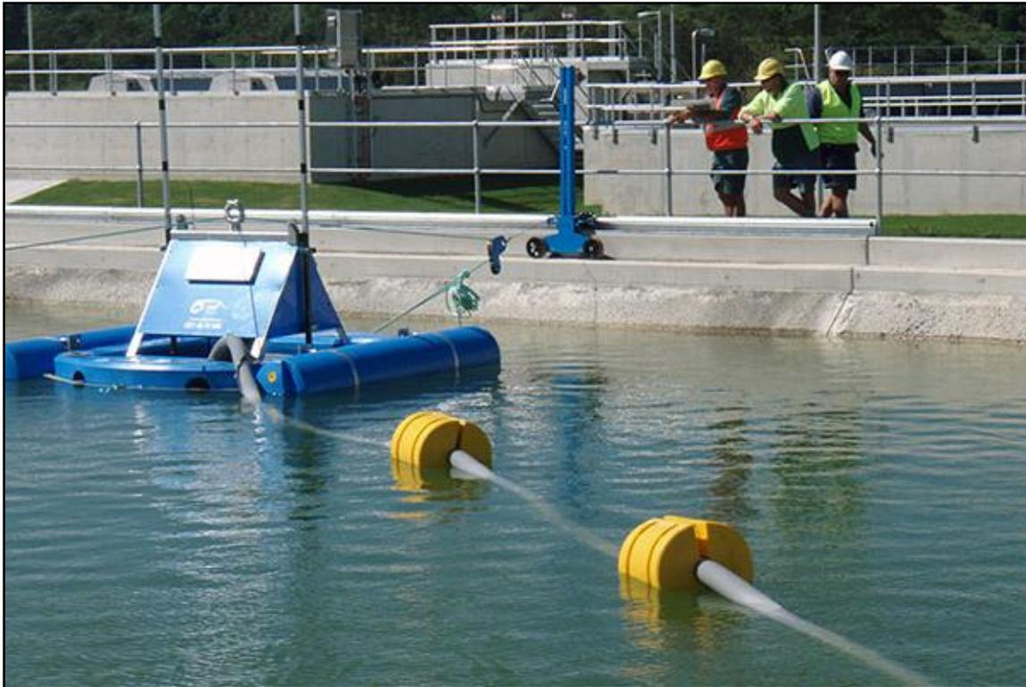
Figure 8-3. Dredge Sled in use (source: Eddy Pump)
