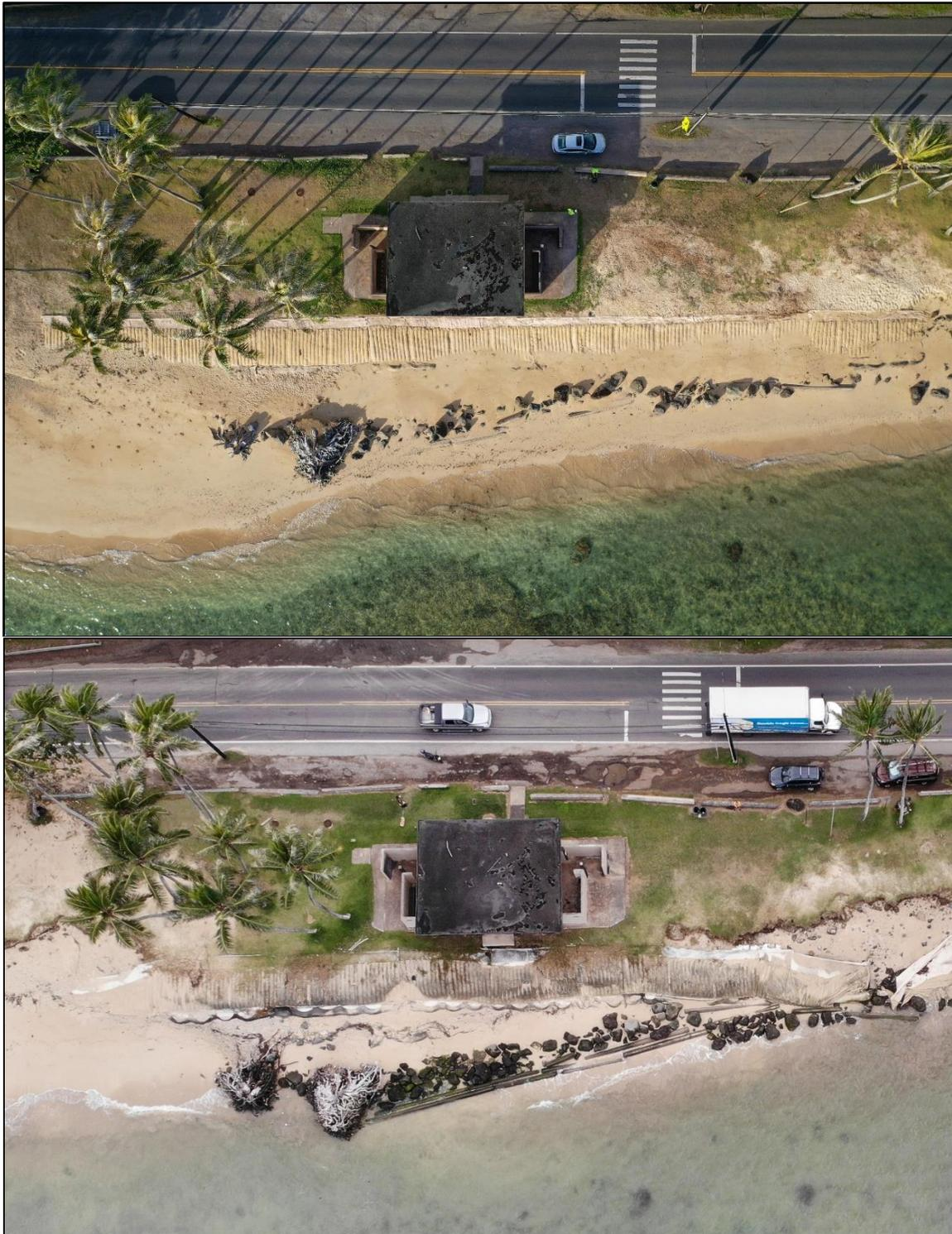
**Figure 4-13. Comparison of temporary erosion after installation in June 2020 (top photo) versus its condition in November 2022 (bottom photo)**
