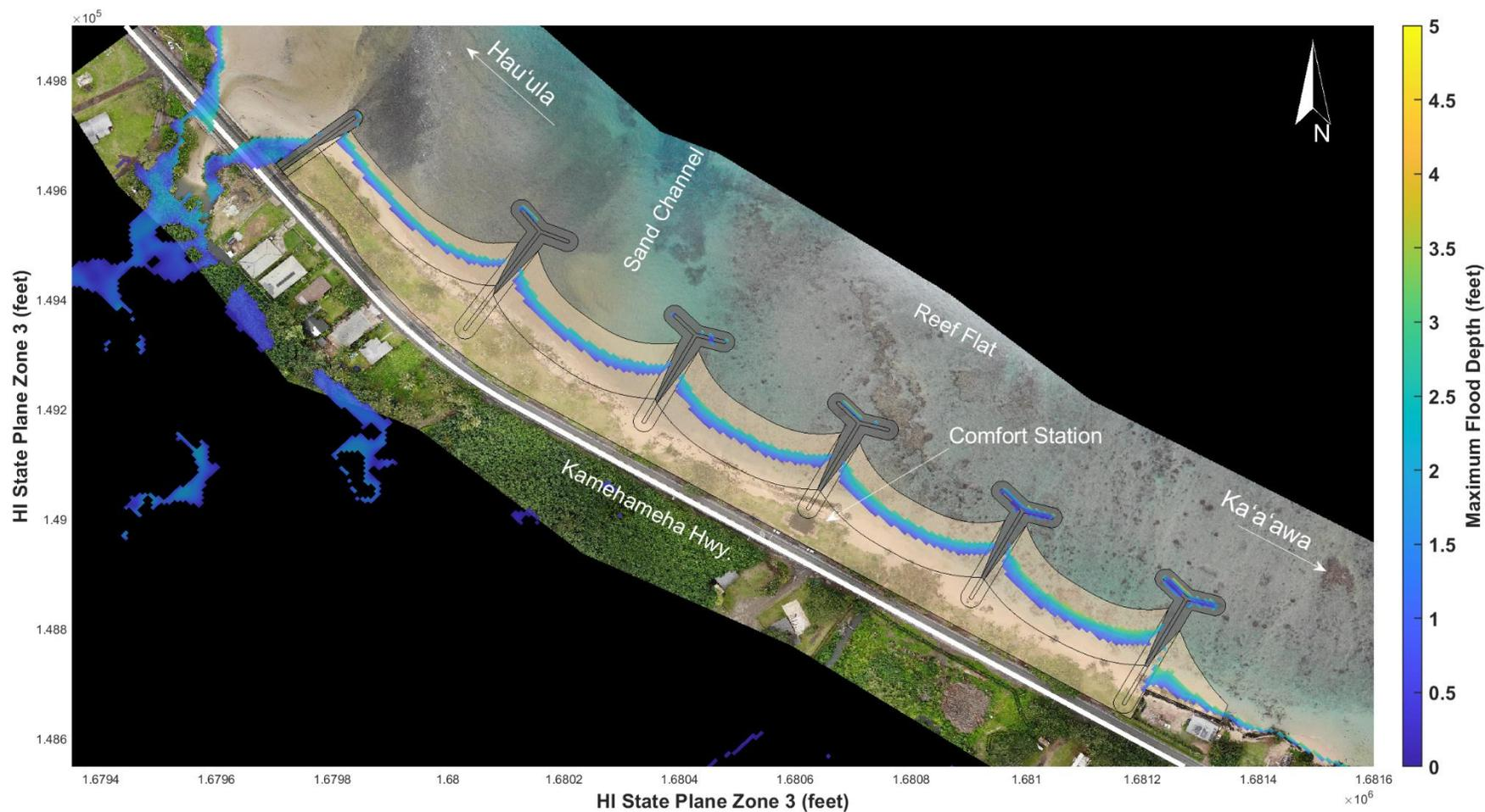
Figure 11-13. Maximum modeled flood depth for stabilized pocket beaches concept with +1.6 ft of SLR during a prevailing wave event
