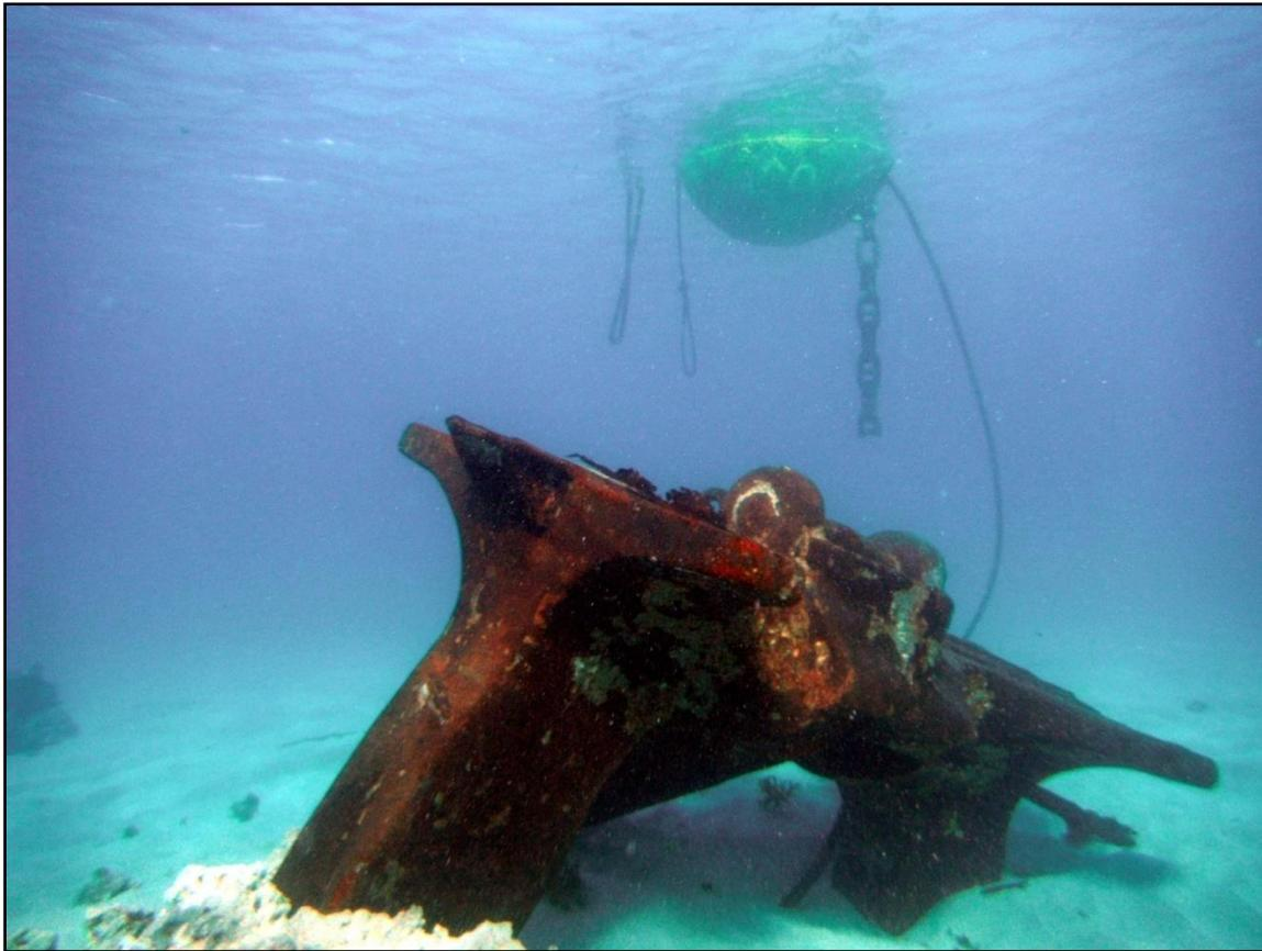
**Figure 8-4. Example: anchor and anchor float used in the 2012 Waikiki Beach Maintenance Project**
