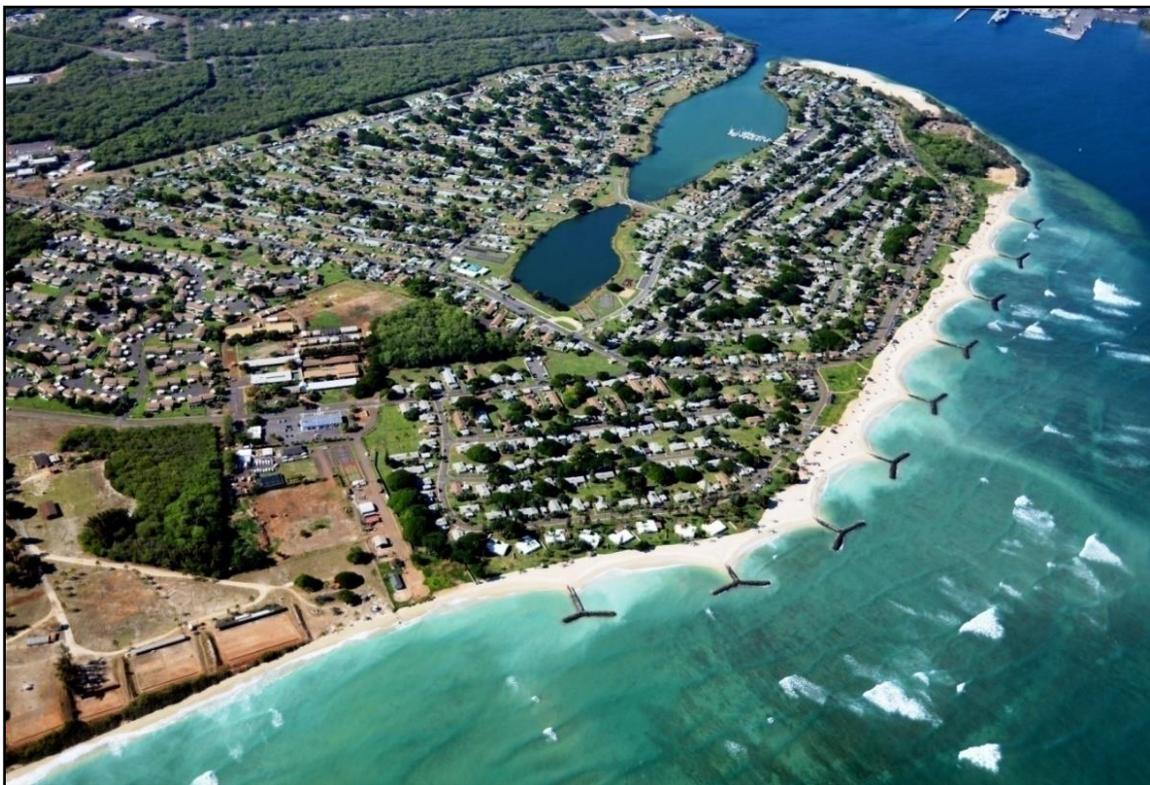
Figure 2-5. Nine rock headland structures stabilize 4,000 ft of sand beach at Iroquois Point
