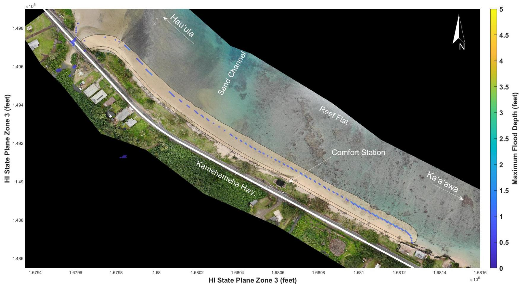
Figure 11-2. Maximum modeled flood depth for the beach nourishment concept for existing sea level during a prevailing wave event
