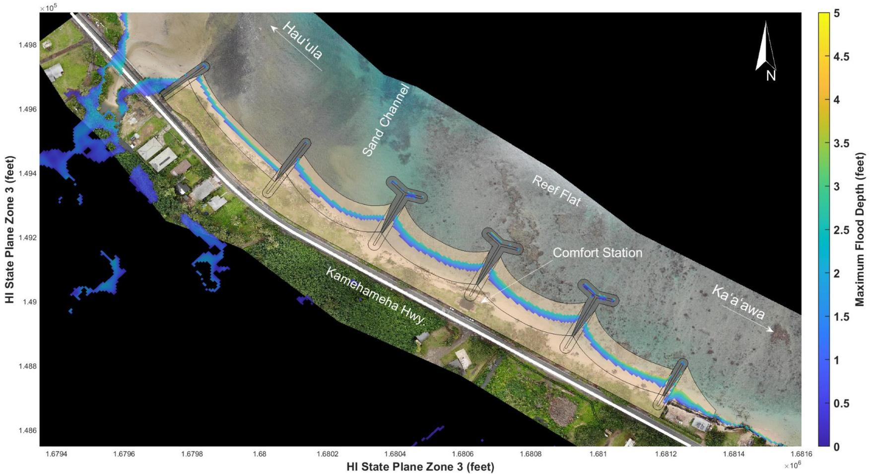
Figure 11-15. Maximum modeled flood depth for the hybrid stabilized pocket beaches concept with +1.6 ft of SLR during a prevailing wave event
