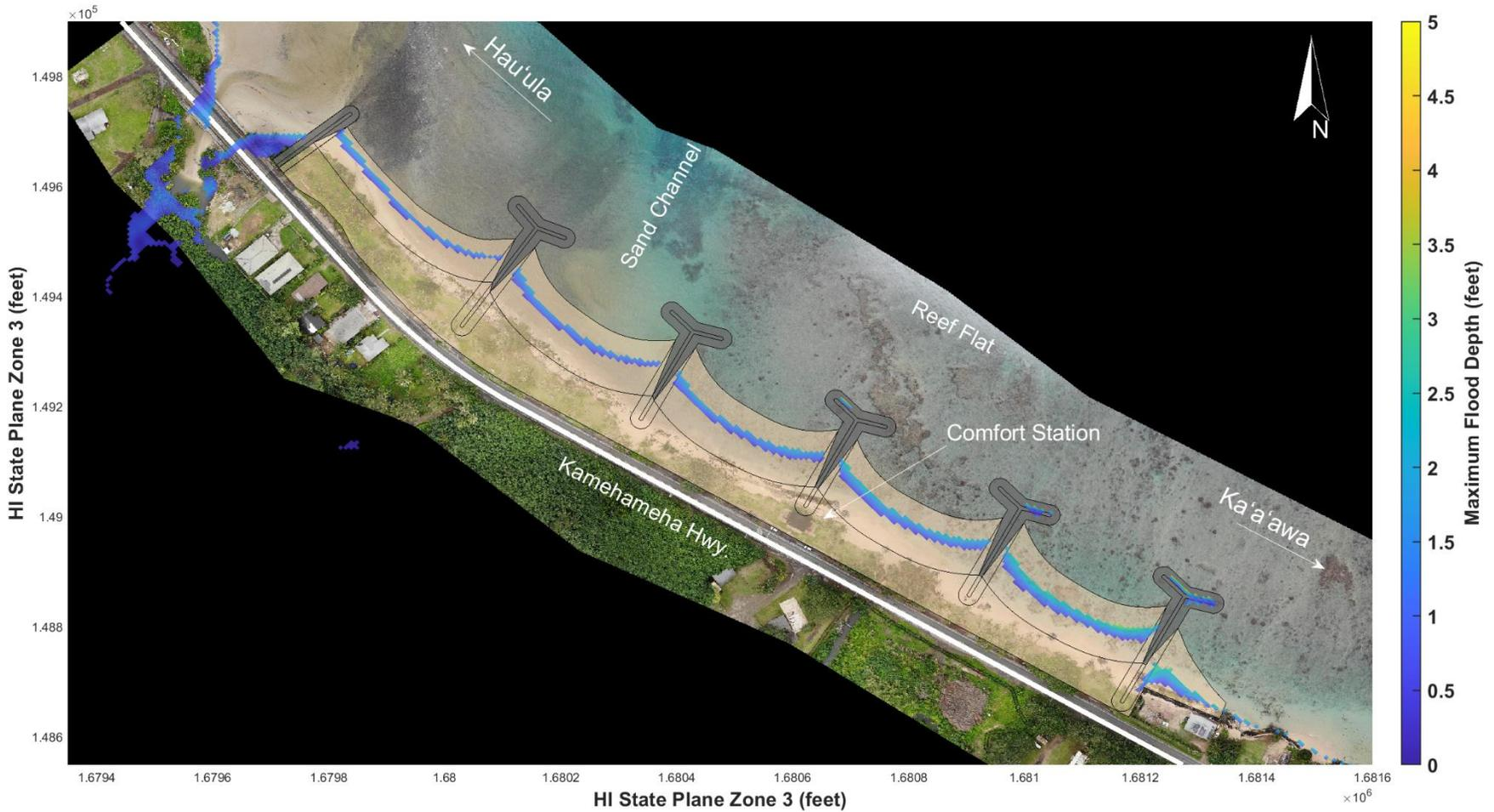
Figure 11-8. Maximum modeled flood depth for stabilized pocket beaches concept for existing sea level during an annual wave event
