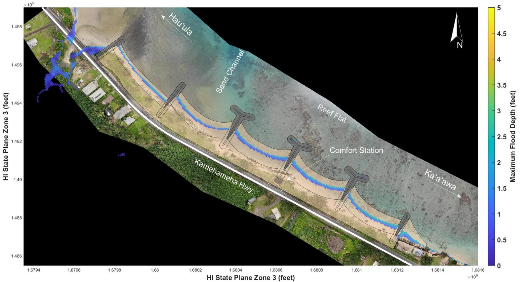
Figure 11-10. Maximum modeled flood depth for the hybrid stabilized pocket beaches concept for existing sea level during an annual wave event
